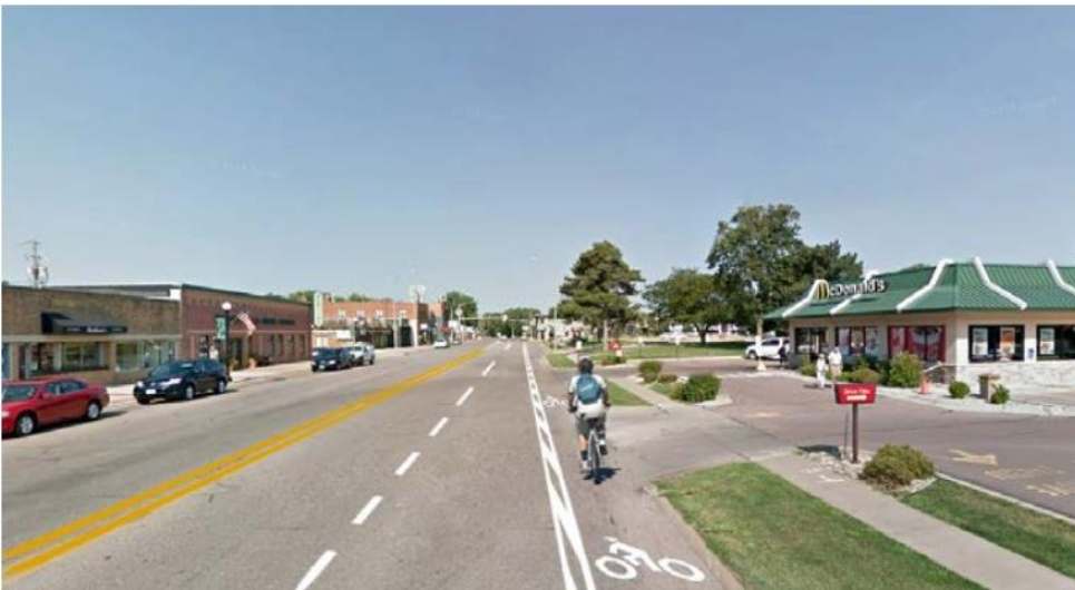
Figure 71. Morningside Ave.: Proposed buffered bike lane.
